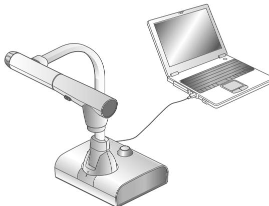
This product is compliant with UVC (USB video class) and troublesome installing of a driver is not required.
